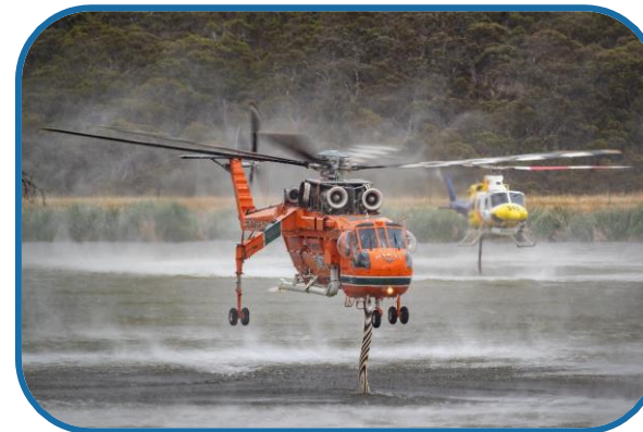
Figure 17. Bundoora, Australia - December 30, 2019: Erickson Air Crane firebombing helicopter (Sikorsky S-64) sucking up water to fill its tank in a lake while a smaller Bell 412 helicopter fills behind. Photo by Ryan Fletcher, Shutterstock.
