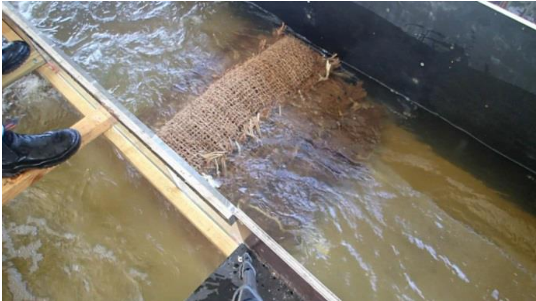
Photo 3.2. Example of wave attacks on oyster filled bags in WRL (Coghlan 2017).
