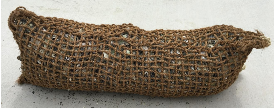
Photo 3.1. Custom-made coir (coconut fibre) bag filled with loose, dead oyster shell.
