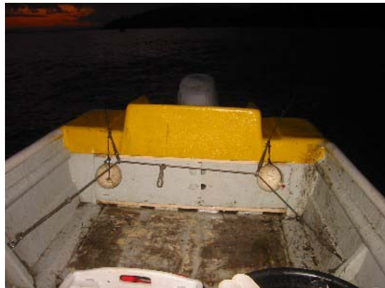
Figure 18 Both hauling ropes are connected to the boat and it continues forward to remove the slack from the hauling ropes and net
