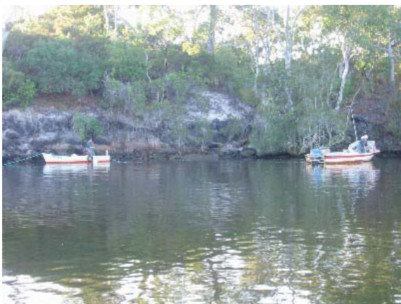
Figure 3 Winch punt is anchored and main boat shoots hauling rope then net
