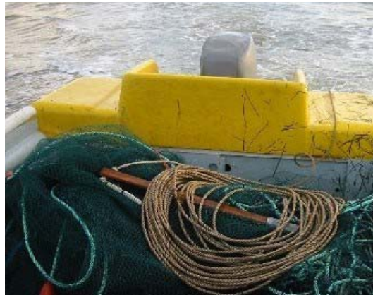
Figure 16 Shooting hauling rope after deploying float at the commencement of the shot
